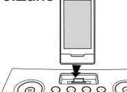
Insert a Zune into the dock with proper insert (Zune must not be in a skin or case). The Zune will charge while docked. Press the MI Button on the ZN90 to play your Zune.
